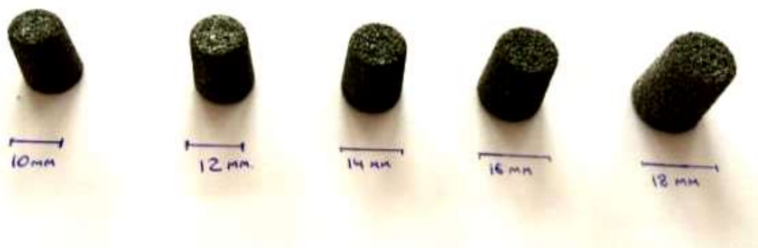
Figure 4 - Porous composite implants made of titanium nickelide for surgical treatment of flatfoot deformity in children of standard shape and sizes.
